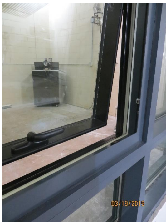
Figure 2 – Operation of operable section of test specimen
