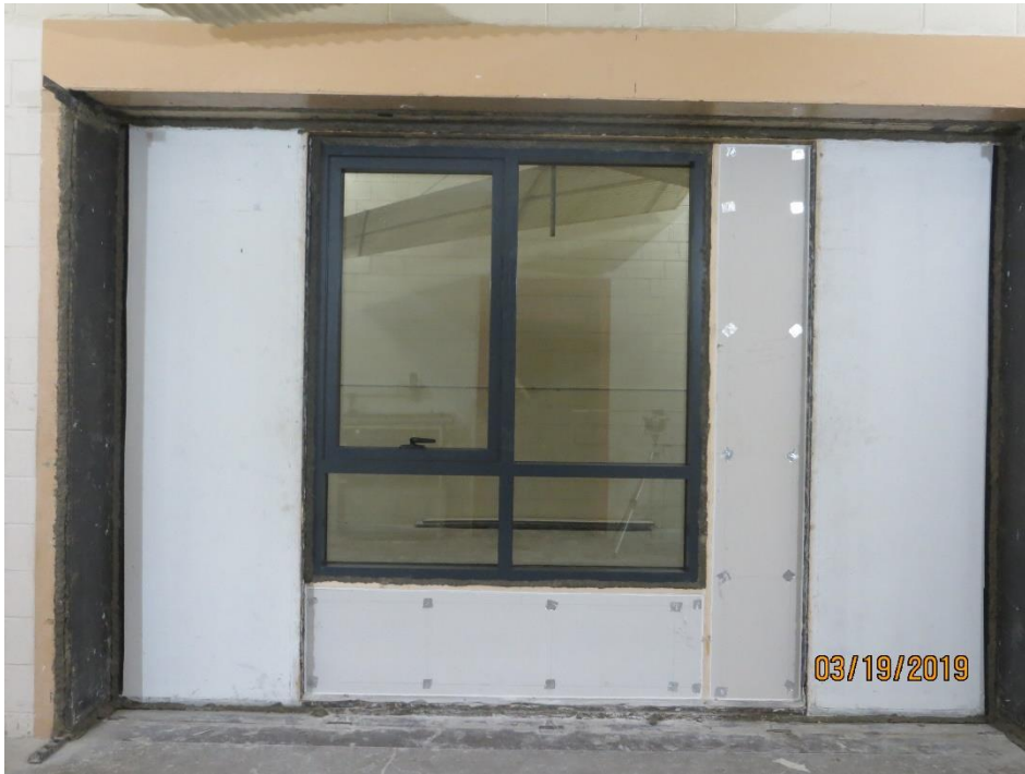
Figure 1 – Specimen mounted in test opening, as viewed from receive room
